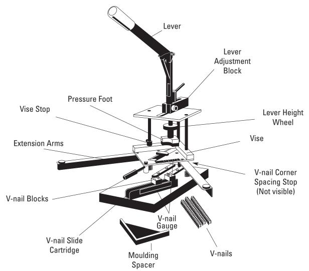
V-nails - Moulding fasteners.
