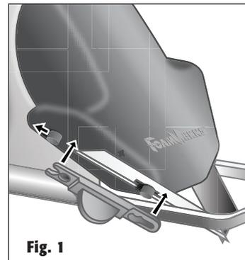
**Blade Storage Drawer** - Located on the rear of the tool, used to store extra blades
