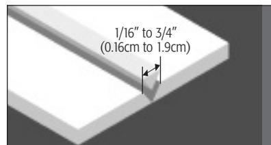
Cuts V-Grooves into foamboard or cellfoam, with resulting V-grooves 1/16" to 3/4" wide (0.16cm to 1.9cm).
