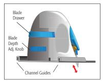
Blade Storage Drawer - Located on the rear of the tool, used to store extra blades
