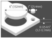
Cuts foamboard or cellfoam circles from 1"to 6" diameters (25.44 to 152mm), and depths from 1/8" to 1/2" (3.2 to 12.7mm).
